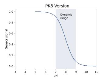
Calibration of both versions is performed at low pH values (completely protonated indicator dye) and at high pH values (completely de-protonated indicator dye). For this reason, it is possible to use the same pH buffer capsules (**PHCAL2** and **PHCAL11**) for both pH sensor versions.
