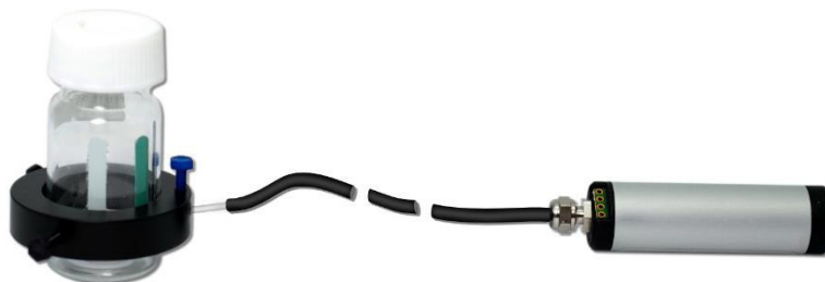
Figure 5: Connection of an oxygen vial to Pico-O2 via an optical fiber.
