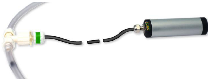
Figure 3: Connection of pH flow-through cell to Pico-pH via an optical fiber.
