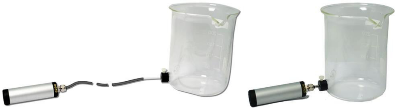
Figure 2: Connection of temperature sensor spots to Pico-T via an optical fiber (left) or a rod (right).
