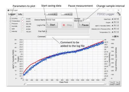
The actual measured parameter is the oxygen partial pressure (hPa) at the sensing membrane. Pressure and humidity sensors are placed inside the FDO2 and these parameters are measured through a venting capillary at the backside of the housing. If the air pressure at the oxygen sensing membrane is identical to the air pressure at the venting capillary (backside of the sensor), the internal pressure can be used for converting the oxygen partial pressure (hPa) into units of %O2.
