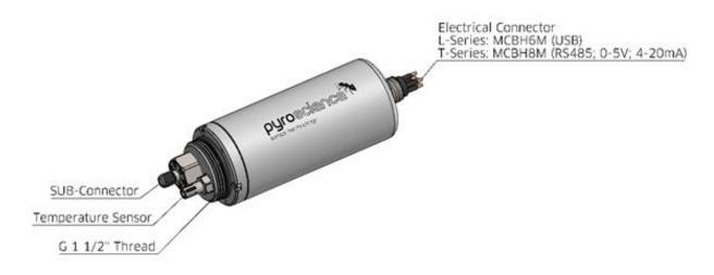
The housing is dependent on the chosen device. **APHOX-TX** comes with a titanium housing for deployments down to 4000m. **APHOX-T-PH** and **APHOX-T-O2** come with a POM housing capable for deployments down to 100m.
