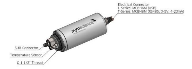
The housing is dependent on the chosen device. APHOX-LX comes with a titanium housing for deployments down to 4000m. APHOX-L-PH and APHOX-L-O2 come with a POM housing capable for deployments down to 100m.
