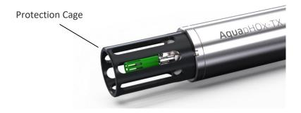
In shallow water environments, it is strongly recommended to slip over the APHOX®-CAP-AF anti-(bio)fouling net onto the sensor cap and to use the APHOX®-CAGE-AF with anti-biofouling net on the APHOX® device (instead the included protection cage).
