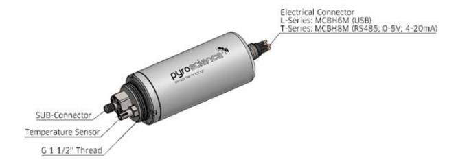
The housing is dependent on the chosen device. APHOX-TX comes with a titanium housing for deployments down to 4000m. APHOX-T-PH and APHOX-T-O2 come with a POM housing capable for deployments down to 100m.
